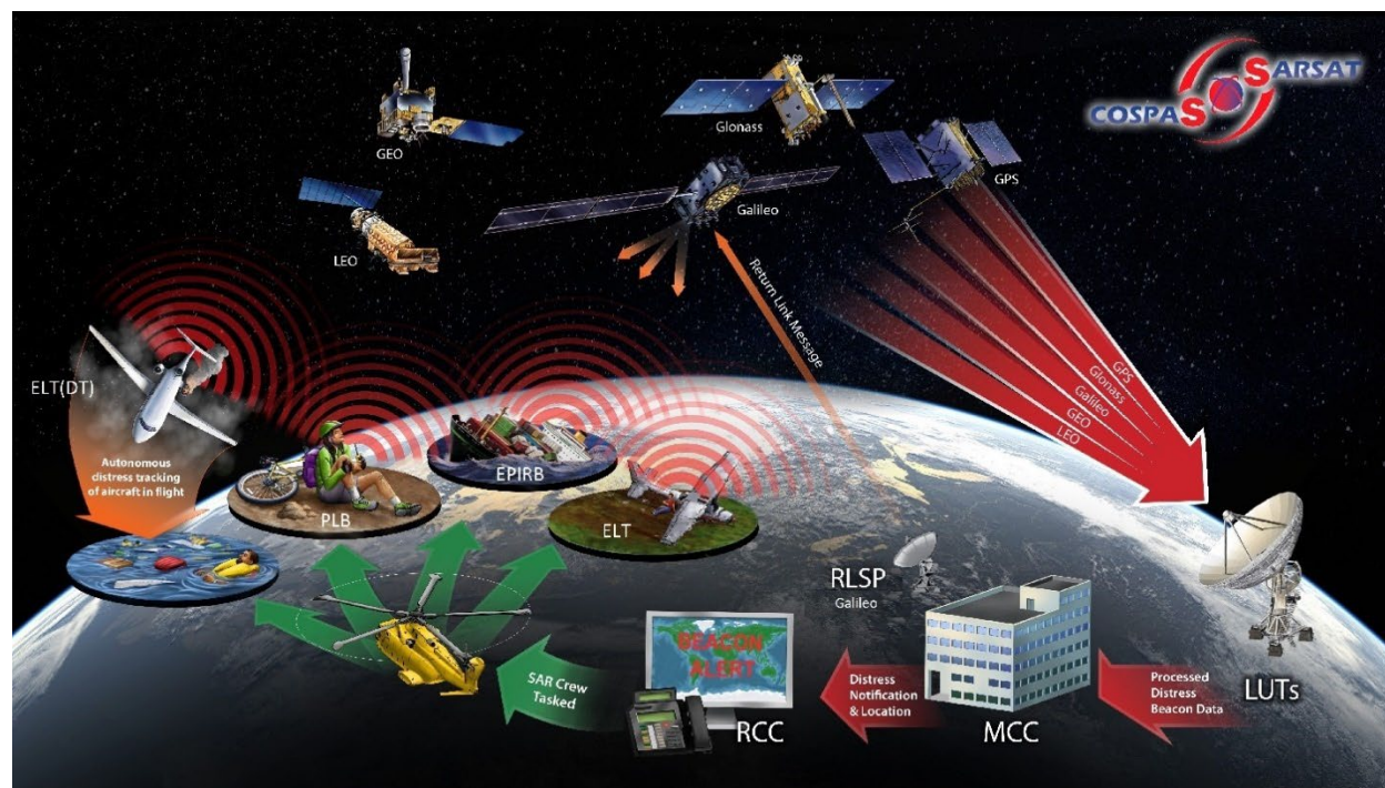
Figure 8: Cospas-Sarsat System Overview
