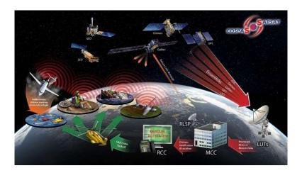
The basic Cospas-Sarsat concept is illustrated in the above figure. The System is composed of:
